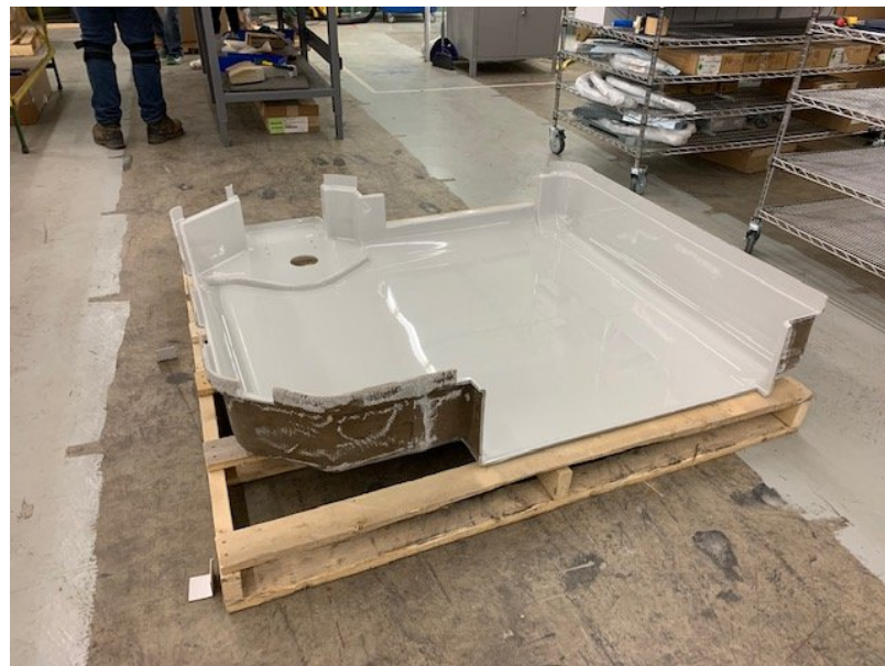
New Restroom Module – Floor Pan
