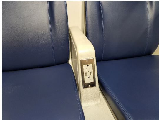
Convenience Outlet Upgrade
